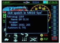
"Home system" can only be MX10 or MX10EC command station or later ZIMO system control centres (see also chapter *CONFIG*, Control centre, *Home system*), but not Roco Z21 or an old ZIMO base unit MX1. Automatic import of GUI or GUI elements from the MX10 into the controller:
