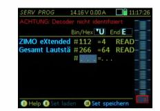
An active shunting mode (R-key engaged) is automatically terminated when calling the CV-programming screen (OP PROG and SERV PROG)!
