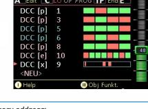
Alternative, quick method of entering a new accessory address: Directly from the operating screen LOCO:
