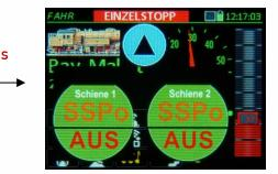
The **S-Key** can also be used as a quick alternative to take over a loco when "External Control" is shown in the header, but the **train IS NOT moving** (i.e. speed slider at 0): Press the **S-Key** (has no effect since the train is already stopped) but the "External Control" is removed and the controller is fully functional (the address is deactivated on the other controller and "External Control" is being displayed there).
