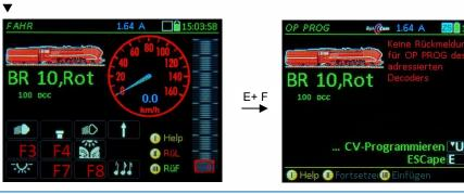
NOTE: **OP PROG** is possible while driving or at standstill. The vehicle can be driven normally while programming or reading out data. Of course, data transmission tends to be worse while driving and it is therefore recommended to drive only when RailCom feedback is available (or the programming changes can be seen instantly by the vehicle's behavior).
