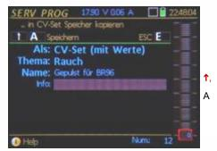
Soft-Key III = Paste...→ Search for the desired CV-Set in the CV-Set database and paste the CV-set rows to the current display screen.
