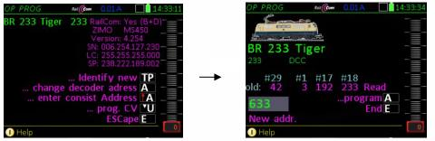
An input field appears under the "Old data", in which  $\blacktriangle$  the new address is entered.
