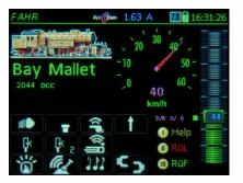
For programming and reading CVs on the main track (Operational Mode = PoM, Programming on the Main); change also decoder address or enter Consist address. i.e in the operational mode *LOCO*, also E + F
