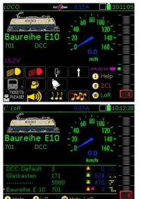
LOCO MOD is a variation of LOCO IN: no new address is entered, but the currently active address is automatically entered in the 'ADDR' field (at the second 'A').
