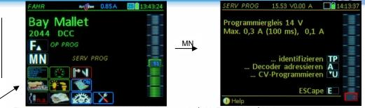
The first screen after entering the *SERV PROG* mode (with E + MN keys) is the programming menu, which also functions as a "security question" to prevent accidental deletion of decoder addresses or data.
