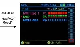
Address 0 ("900") should NOT be appointed for operational purposes!! To actually address the MX9 (from 0 to the target address) again: Softkey III  $\rightarrow$  Open the "Object menu" for the same MX9
