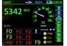
After approx. 0.2 seconds (with undisturbed transmission, otherwise slower), the first data has already arrived. Information for image, selected speedometer disc and name; however, the function icons are still missing, which - depending on the number - account for the majority of the data volume to be transmitted.
