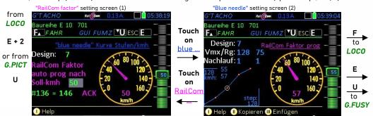
The correct setting of the "blue needle" curve is highly recommended (e.g. due to the future necessity for ETCS operation). This is done quickly and easily by moving to the individual support points using the slider (marking) and then transferring the current RailCom-reported speed to the centre of the speedometer disc by touch (after "settling").
