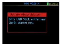
After the update, the **prompt to remove the USB stick** is displayed, followed (always) by an **automatic reset** and start-up of the MX33.
