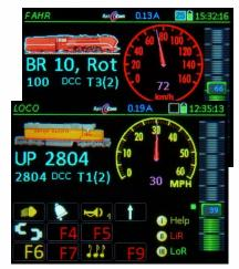
If an address in the *LoR* is marked with "FT (..)", the vehicle can not be activated directly because it is part of a consist in another controller \*), which is NOT ACTIVE at the moment (not in that controller's foreground). If, on the other hand, this consist is currently ACTIVE in the other controller (i.e. one of the vehicles involved is in the foreground on that controller), "FS (..)" is displayed in the *LoR* (= external control with the number of consisted vehicles).
