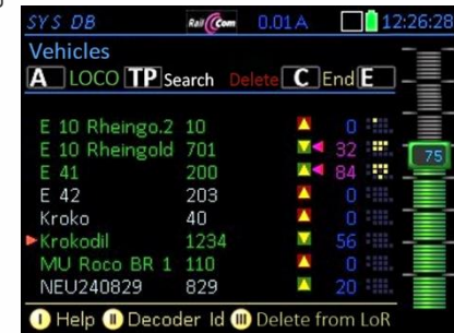
By activating it (using the A button from the SYS DB, grey line), the screen LOCO is opened for the address, and it is also entered into the LOCO DB and LoR i.e. green line in the screen 'SYS DB'
