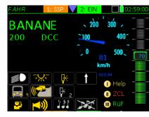
When the STOP Bullets are replaced by the small blue arrow in the header (pointing down): <u>Touching the small blue arrow</u> (in the header) → reopens the "STOP Bullets"
