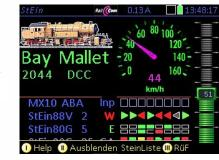
In this example, there are several StEin modules in the list, two of which just show the turnout positions and the other track sections with different HLU and east-west states.
