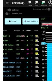
Bv activating it (usina the A button from the SYS DB, grey line), the screen LOCO is opened for the address. and it is also entered into the LOCO DB and LoR i.e. green line in the screen 'SYS DB'
